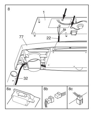
9. Securely tighten a plastic tie around the Wire Harness (22) and under the indicated hook on the Console (1) to prevent the Wire Harness from slipping. Tighten the plastic tie and cut off the end.
